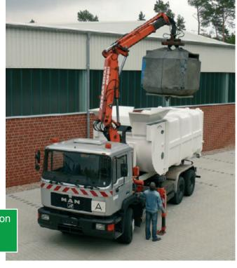
Special design for operation on truck, with low construction height and loading funnel
